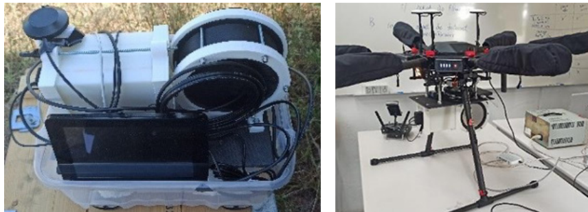
Figure 4. Developed handheld equipment (left image) and radiation detection system integrated in a multirotor DJI Matrice 600 Pro (right image) [5].
