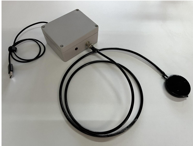
Figure 5. The final device, consisting of the waterproof sensor and the electronics enclosure.
