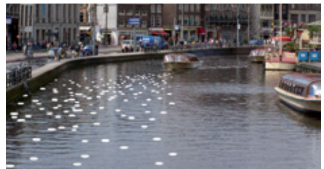
Artistic illustration of exploited prior knowledge in the EKSPLORE project. The future path of the boat is predicted by a particle filter (illustrated by the disks on the water) taking into consideration the prior knowledge of the water lane.
