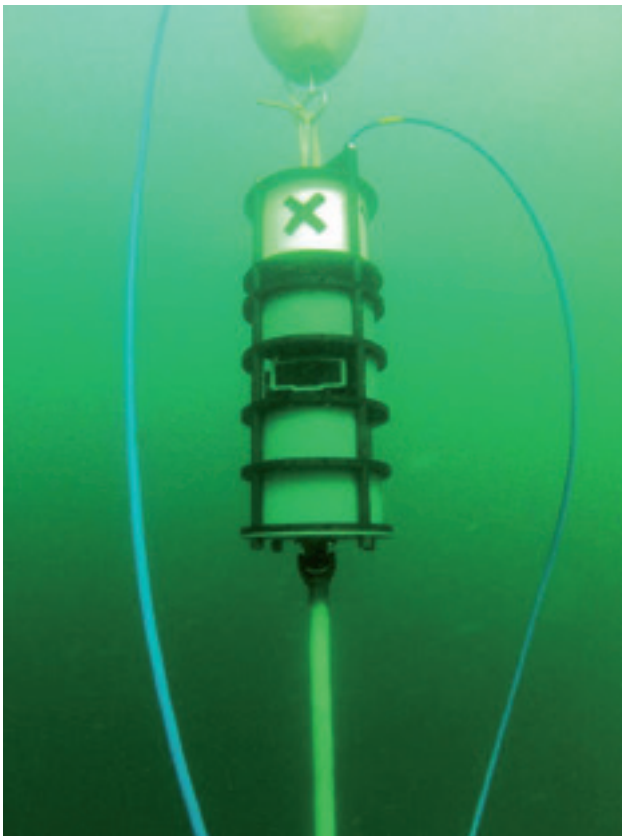
A diver detection sonar in a HAPS (Harbour and Base Protection Systems) sea trial
