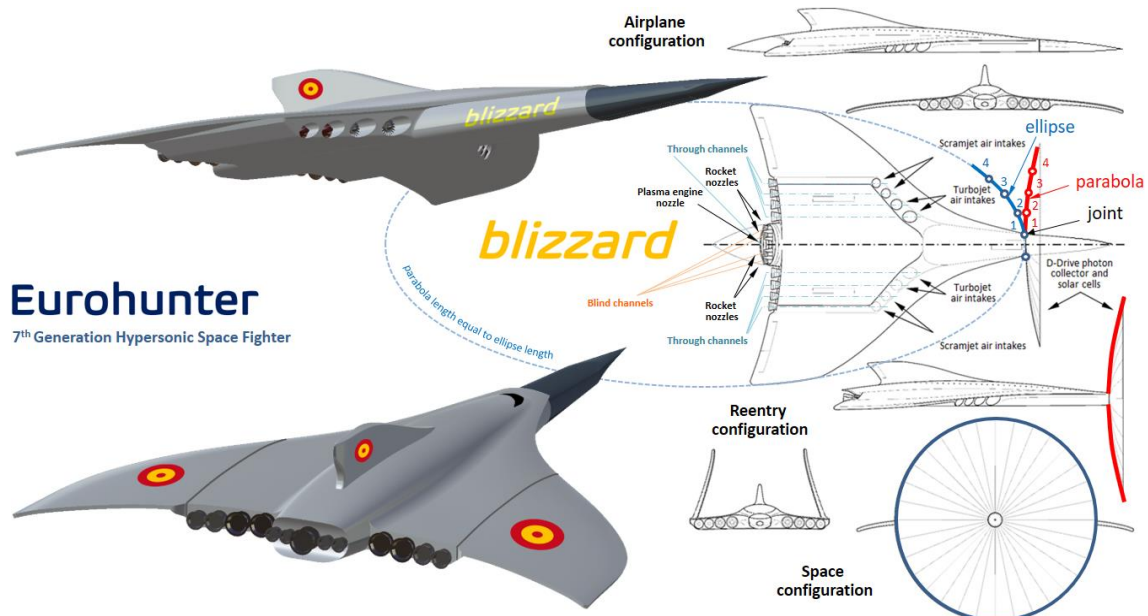
Figure 1. Blue prints and 3D views of the three configurations (airplane, space and reentry) of the 7th Generation Eurohunter Blizzard multirole fighter and space defender.
