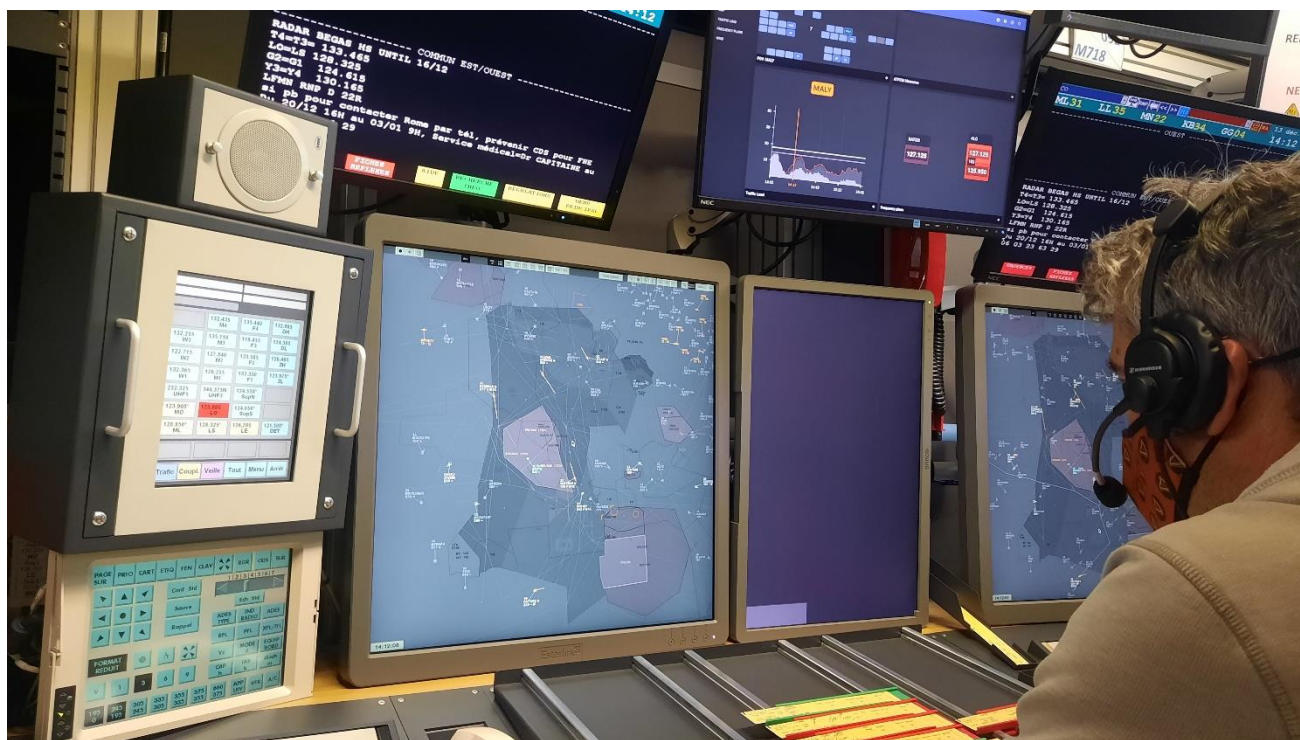
Fig 5: The screen above the radar scope shows the traffic density in the control sector
