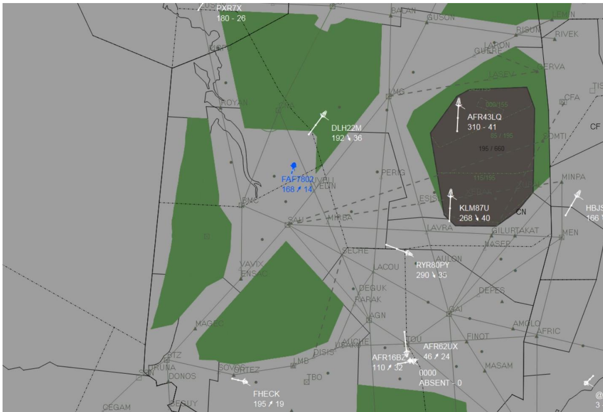
Radar screen shot- FAF 7802 initial Climb, crossing FL 168 up to FL 180, controlled by Bordeaux
