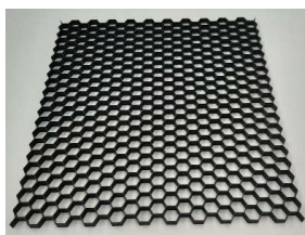
Figure 2. AM Radar absorbing honeycomb. NLR.
