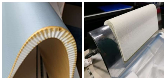
Figure 1. Additive manufactured honeycomb surface (left) and the tool to co-cure resin skin on to the core (right). AM absorbers on the rear base plate is not shown. Saab.
