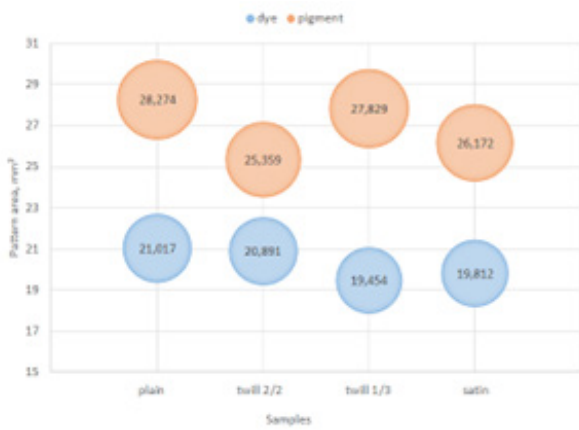
Figure 2: Change in the surface of printed motifs on different fabric weaves
