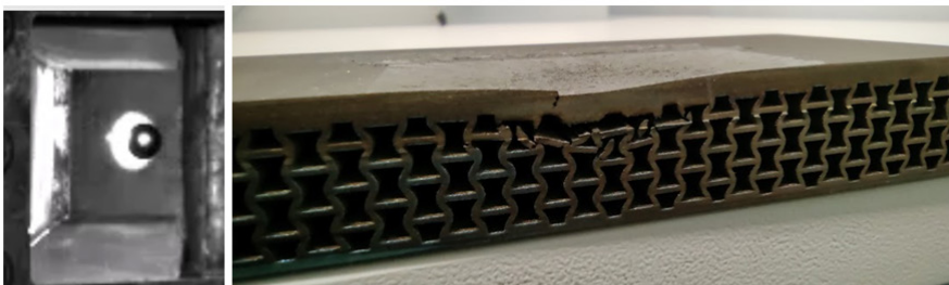
Figure 2. Left: Composite test specimen (titanium reticular matrix + CSi tile) in the very moment of a high velocity impact (9g, 13 mm solid steel bearing, 864 m/s impact). Right: titanium matrix after impact.
