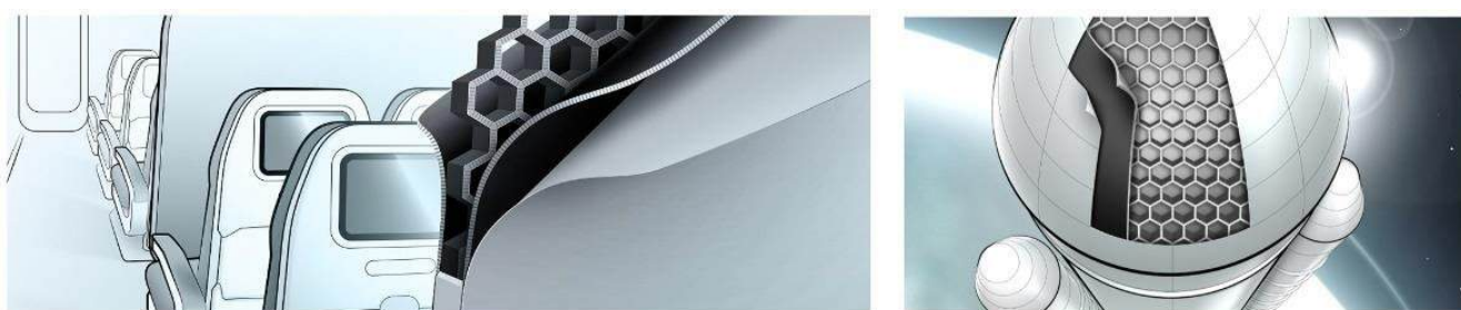
Fig. 2 Potential applications of hierarchical sandwich honeycombs with sandwich skins (left: aircraft interior wall, right: nose fairing structure in a space launcher).
