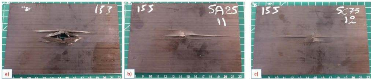
Fig. 1 CFRP laminates post-impact with coatings removed, where present. a) reference laminate, b) 25%SSG and c) 75% SSG content.
