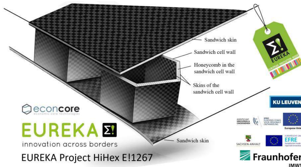
Fig. 1: Hierarchical honeycomb structure with honeycomb cores within the sandwich cell walls and within the sandwich skins.
