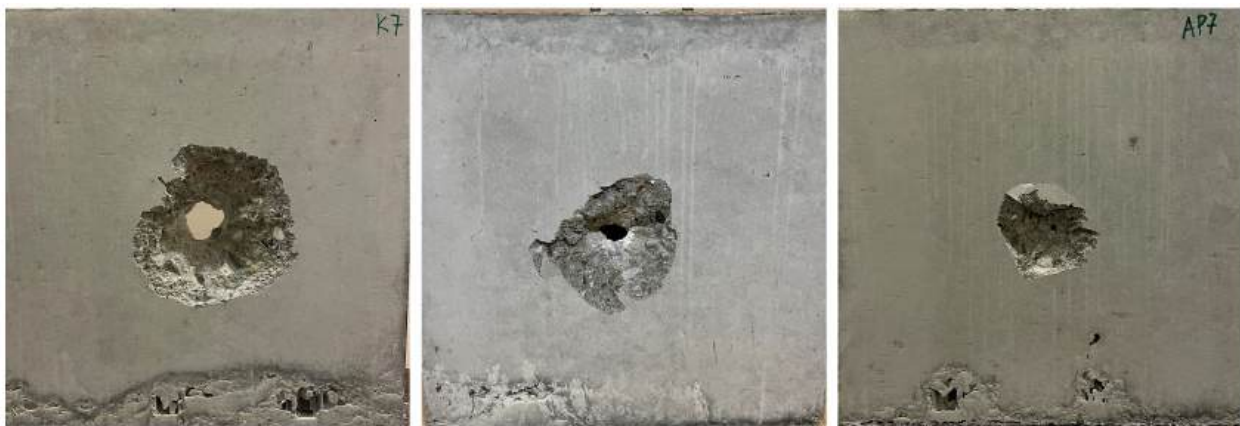
Fig. 2 Scabbing craters on three concrete plates at approximately the same impact velocity, v_i : (a) ball bearing at 641 m/s; (b) FSP at 634 m/s, and (c) AP core at 676 m/s.
