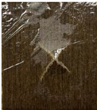
Fig. 3 Tested flax fibre reinforced skin sandwich plate.
