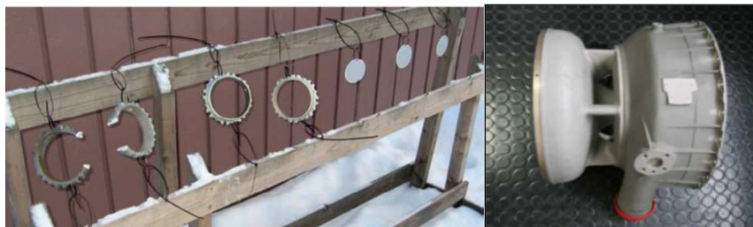
Example of landing gear pieces in 300M steel and A357 aluminum air intake developed in the ECOCOAT project.
