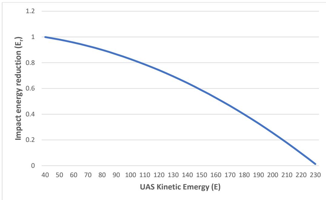
Figure 18: Quadratic relationship between the  $E_r$  and  $E$  at impact
