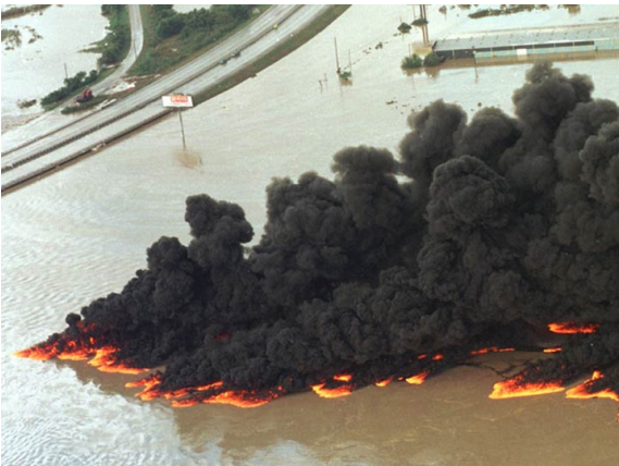
Figure 2 Flooding in the San Jacinto river basin led to the rupture of oil pipelines which spewed flammable hydrocarbons into the floodwaters where they ignited. Photo credit: USGS
