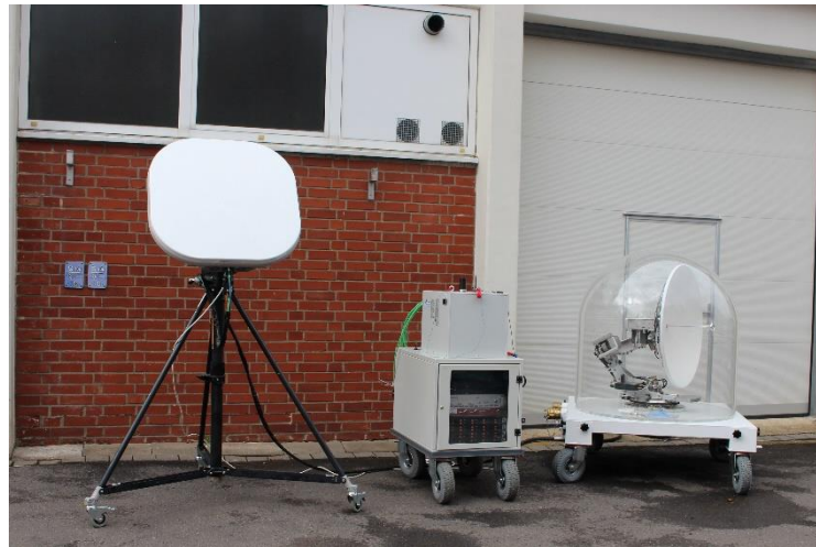
Figure 22: Potential setup for the SABBIA® system. In this case, one electronically steerable antenna is used for reference signal acquisition, and one mechanically steerable antenna is connected to the receiving channel. The RF-front end is hosted in the case in the center.
