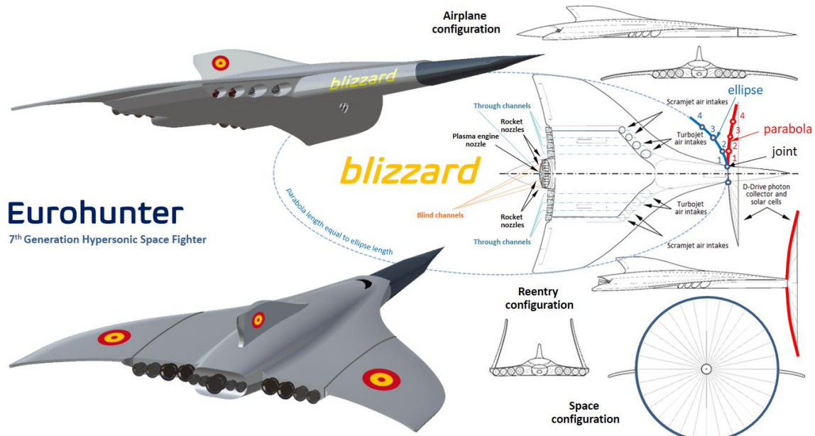
Figure 1. Blue prints and 3D views of the three configurations (airplane, space and reentry) of the 7th Generation Eurohunter Blizzard multirole fighter and space defender.
