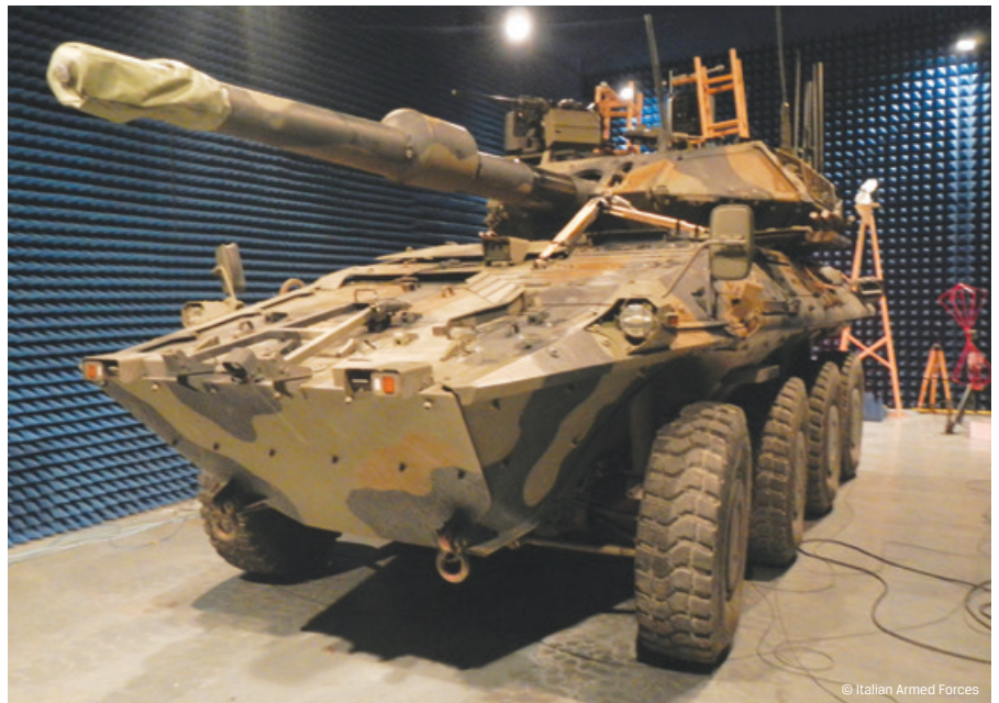
The Centauro II vehicle undergoes electromagnetic compatibility tests ensuring performance and safety at the Army Multifunctional Experimentation Centre in Cepolispe, Italy.
