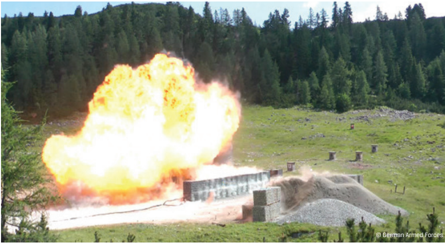
The Bundeswehr Technical Center for Protective and Special Technologies in Oberjettenberg, Germany, carries out a blasting test on a Vehicle Borne Improvised Explosive Device (VBIED).
