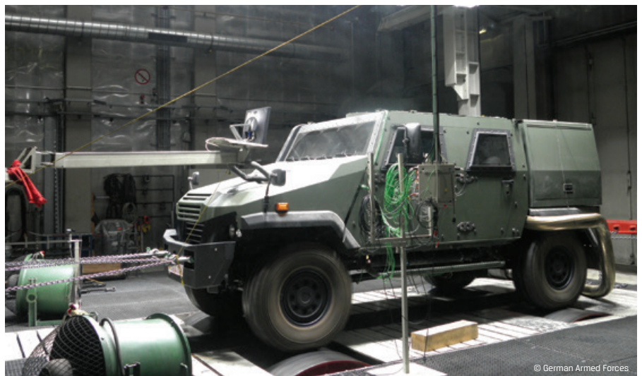
The Bundeswehr Technical Center for Land-Based Vehicle Systems, Engineer and General Field Equipment in Trier, Germany, tests the MOWAG EAGLE V armored vehicle on the roller bench.
