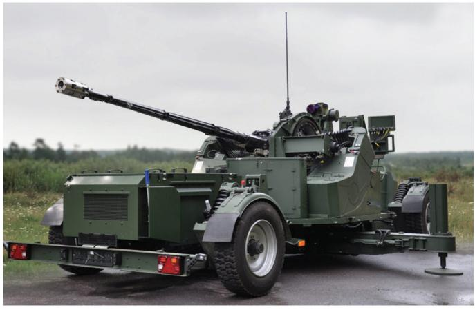
A PGZ photo shows a SA-35 anti-aircraft gun. SA-35 is a 35mm automatic gun mounted on a truck chassis, designed entirely by Polish engineers.
