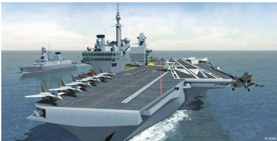
PA2 was a planned aircraft carrier under development by Thales Naval France and DCNS for the French Navy
