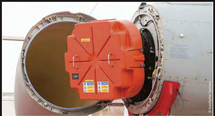
Eurofighter's new CAPTOR active electronically scanned array radar
