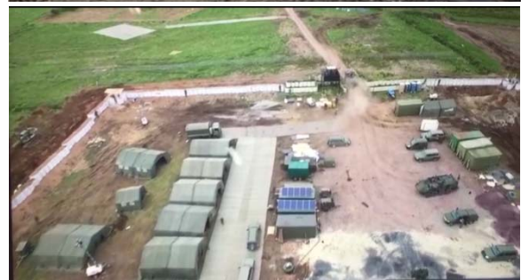
Solar PV on Irish DF Deployed Kitchen Unit
