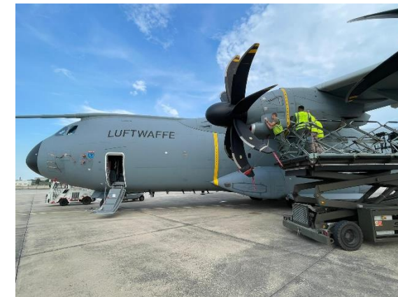
Spanish, French and Belgian technicians perform oil refueling on DE A400M
