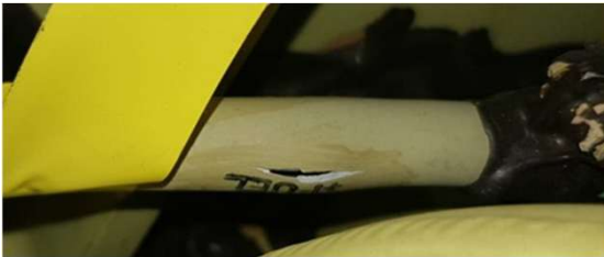
Cracked fuel pipe
