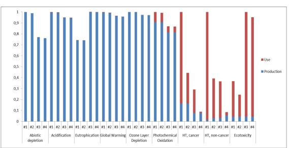
Figure 1. Life-Cycle impact comparison between the four 9 mm ammunitions: #1 – steel-lead projectile with lead primer; #2 – steel-lead projectile with non-lead primer; #3 – composite projectile with lead primer; #4 – composite projectile with non-lead primer
