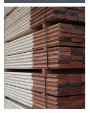
In the past, Rotterdam used tropical hardwood in all its waterworks, as it is resistant to all types of weather conditions. However, the part of a structure that is under water will never rot. That means it is possible to do things differently. Thanks to a special adhesive technique, it is also possible to use cheaper Dutch softwood.
