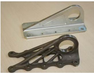
An element as apparently insignificant as a nacelle hinge bracket is the perfect example of additive manufacturing being able to significantly improve existing products. In this case, a combined project between EOS and Airbus (EADS) led to a redesign that not only was able to achieve a reduction in weight and a change of material for this part (from steel to titanium), but also to reduce the overall cost.
