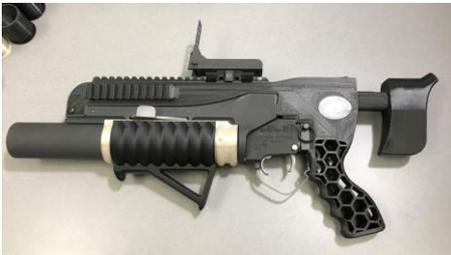
RAMBO is an acronym for Rapid Additively Manufactured Ballistics Ordnance, the result of a six-month project that led to a prototype of grenade launcher similar to the US Army's M203. All 50 parts of the gun, with the exception of the springs and the fasteners, were 3D printed out of steel, aluminium and other materials. The ammunition used in the later test was also 3D printed, obtaining a performance similar to the serial model.
