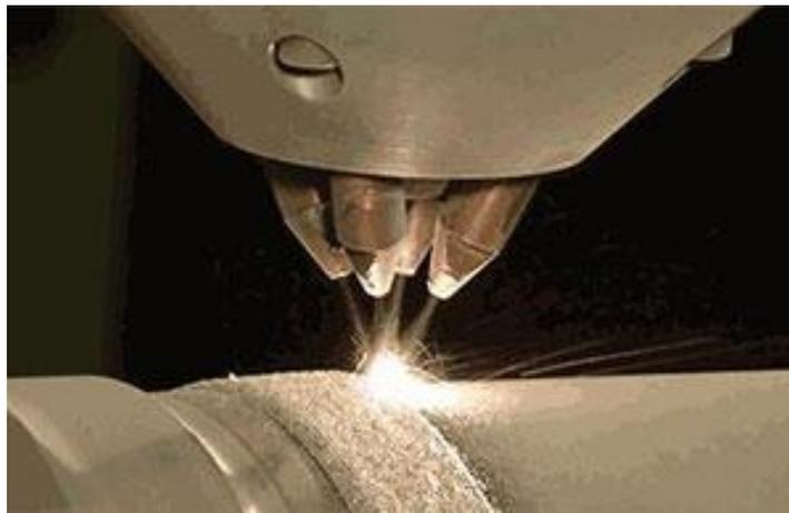
Figure 20: Part being manufactured using LENS AM technology (image courtesy of OPTOMEC)
