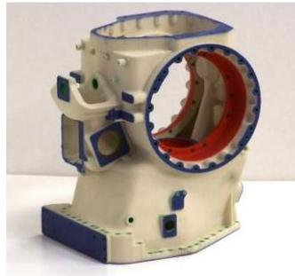
Figure 36: Example of a part produced with BJ technology (image courtesy of Fundación Pro dintec)
