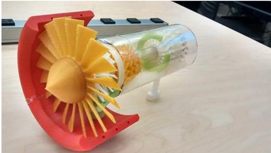
Figure 18: Example of a part produced with FDM technology (Image by C Mitchell under Creative Commons CCBY-SA 4.0. licence, via Wikimedia Commons)
