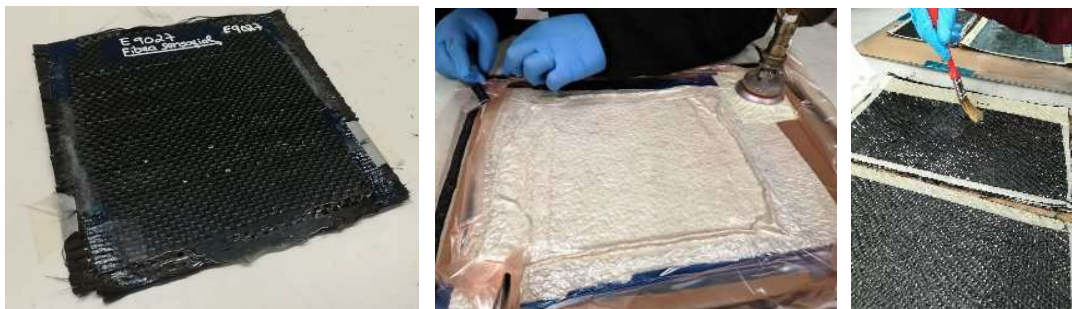
Fig. 5: Details of composite manufacturing stages and obtained composite
