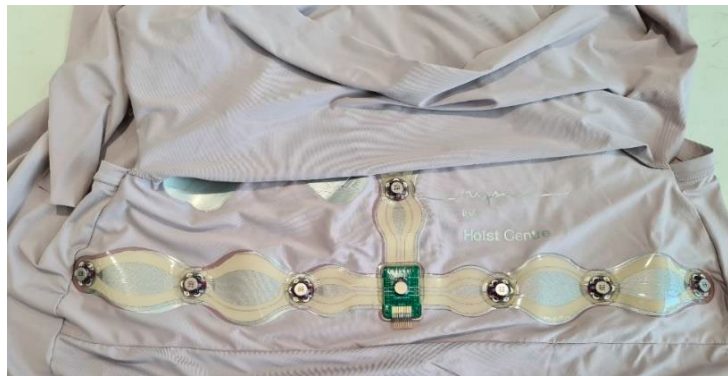
Figure 2. Vibration motors and printed electronics circuitry seamlessly integrated on the fabrics.
