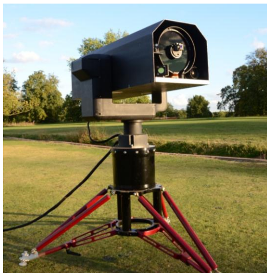
Figure 2: The current HLIN system mounted on a pan-and-tilt head and used during outside stand-off measurements.
