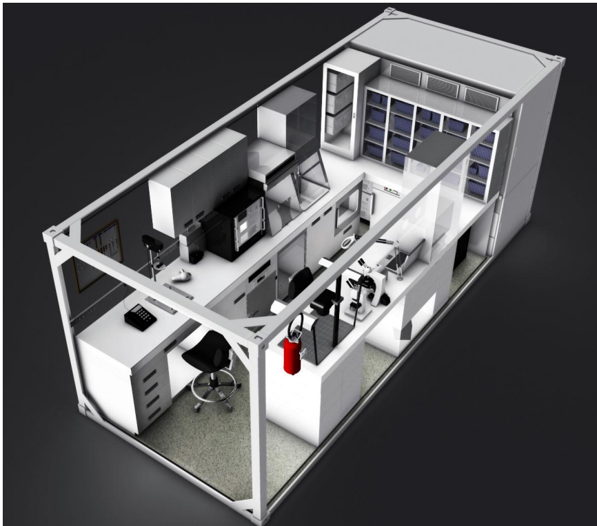
Figure 5: Mobile C-IED Level 2 Laboratory design
