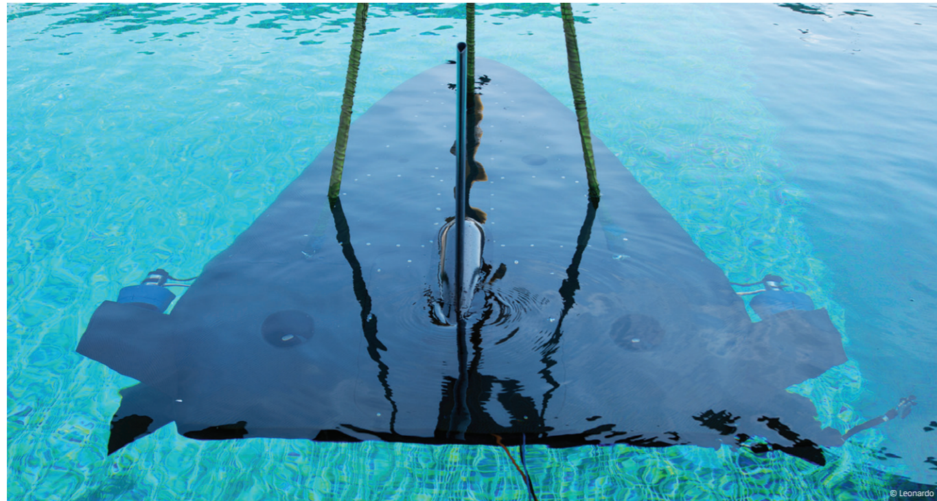
Leonardo V-Fides wire-guidable vehicle for underwater identification & detection used both as ROV (Remote Operated Vehicle) and AUV (Autonomous Underwater Vehicle)
